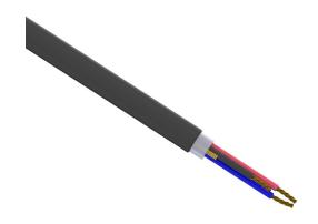
Southwire control cable, unshielded, 3 conductors, 10 AWG, bare copper, PVC/Nylon conductor insulation material, method 1 table 2 color code, PVC jacket, black, cut to length.
