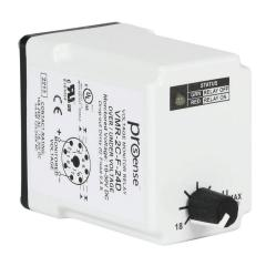
ProSense voltage monitor relay, 1-phase, socket mount, finger-safe, 18-30 VDC input voltage, DPDT, 10A contact rating, 8-pin, LED indicator(s), overvoltage, undervoltage and fixed drop-out protection.
