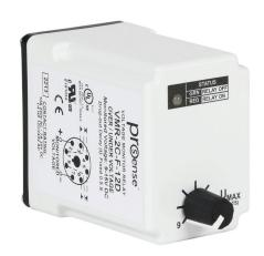
ProSense voltage monitor relay, 1-phase, socket mount, fingersafe, 9-15 VDC input voltage, DPDT, 10A contact rating, 8-pin, LED indicator(s), overvoltage, undervoltage and fixed drop-out protection.
