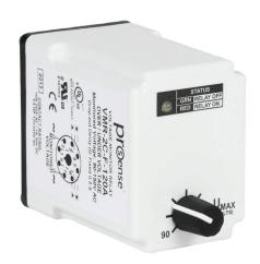
ProSense voltage monitor relay, 1-phase, socket mount, 90-150 VAC input voltage, DPDT, 10A contact rating, 8-pin, LED indicator(s), overvoltage, undervoltage and fixed drop-out protection.
