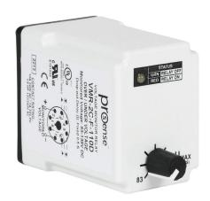
ProSense voltage monitor relay, 1-phase, socket mount, finger-safe, 83-138 VDC input voltage, DPDT, 10A contact rating, 8-pin, LED indicator(s), overvoltage, undervoltage and fixed drop-out protection.
