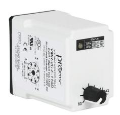
ProSense voltage monitor relay, 1-phase, socket mount, 83-138 VDC input voltage, DPDT, 10A contact rating, 8-pin, LED indicator(s), overvoltage, undervoltage and fixed drop-out protection.
