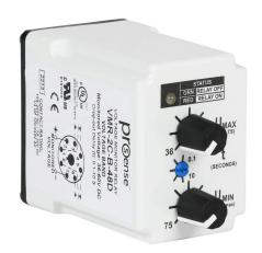
ProSense voltage monitor relay, 1-phase, socket mount, fingersafe, 36-60 VDC input voltage, DPDT, 10A contact rating, 8-pin, LED indicator(s), voltage band protection.
