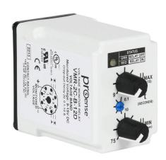
ProSense voltage monitor relay, 1-phase, socket mount, 9-15 VDC input voltage, DPDT, 10A contact rating, 8-pin, LED indicator(s), voltage band protection.
