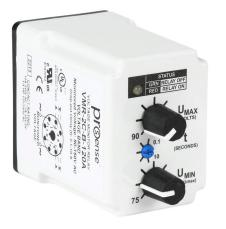
ProSense voltage monitor relay, 1-phase, socket mount, 90-150 VAC input voltage, DPDT, 10A contact rating, 8-pin, LED indicator(s), voltage band protection.
