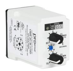
ProSense voltage monitor relay, 1-phase, socket mount, 83-138 VDC input voltage, DPDT, 10A contact rating, 8-pin, LED indicator(s), voltage band protection.
