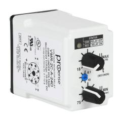
ProSense voltage monitor relay, 1-phase, socket mount, 18-30 VDC input voltage, DPDT, 10A contact rating, 8-pin, LED indicator(s), overvoltage, undervoltage and adjustable drop-out protection.
