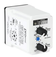
ProSense voltage monitor relay, 1-phase, socket mount, 90-150 VAC input voltage, DPDT, 10A contact rating, 8-pin, LED indicator(s), overvoltage, undervoltage and adjustable drop-out protection.
