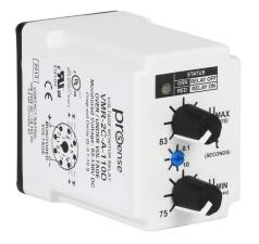
ProSense voltage monitor relay, 1-phase, socket mount, 83-138 VDC input voltage, DPDT, 10A contact rating, 8-pin, LED indicator(s), overvoltage, undervoltage and adjustable drop-out protection.
