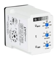
ProSense voltage monitor relay, 1-phase, socket mount, 360-600 VAC input voltage, SPDT, 10A contact rating, 8-pin, LED indicator(s), overvoltage, undervoltage and adjustable drop-out protection.
