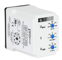
ProSense voltage monitor relay, 1-phase, socket mount, fingersafe, 180-300 VAC input voltage, SPDT, 10A contact rating, 8-pin, LED indicator(s), overvoltage, undervoltage and adjustable dropout protection.
