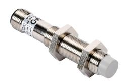
Micro Detectors inductive proximity sensor, tubular, 12mm diameter x 65mm body, nickel-plated brass housing, N.O. output, 4mm sensing distance, non-flush, 25 Hz switching frequency, IP67, 4-pin M12 quick-disconnect.
