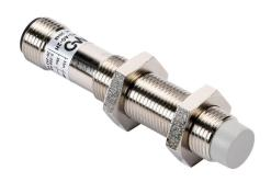
Micro Detectors inductive proximity sensor, tubular, 12mm diameter x 65mm body, nickel-plated brass housing, N.O. output, 4mm sensing distance, non-flush, 25 Hz switching frequency, IP67, 4-pin M12 quick-disconnect.
