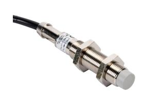
Micro Detectors inductive proximity sensor, tubular, 12mm diameter x 72mm body, nickel-plated brass housing, N.O. output, 4mm sensing distance, non-flush, 25 Hz switching frequency, IP67, pigtail.
