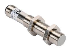
Micro Detectors inductive proximity sensor, tubular, 12mm diameter x 65mm body, nickel-plated brass housing, N.O. output, 2mm sensing distance, flush, 25 Hz switching frequency, IP67, 4-pin M12 quick-disconnect.
