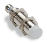
Micro Detectors inductive proximity sensor, tubular, 18mm diameter x 74mm body, nickel-plated brass housing, N.O. output, 8mm sensing distance, non-flush, 25 Hz switching frequency, IP67, 4-pin M12 quick-disconnect.
