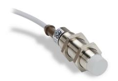
Micro Detectors inductive proximity sensor, tubular, 18mm diameter x 60mm body, nickel-plated brass housing, N.O. output, 8mm sensing distance, non-flush, 25 Hz switching frequency, IP67, pigtail.
