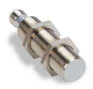
Micro Detectors inductive proximity sensor, tubular, 18mm diameter x 74mm body, nickel-plated brass housing, N.O. output, 5mm sensing distance, flush, 25 Hz switching frequency, IP67, 4-pin M12 quick-disconnect.
