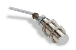
Micro Detectors inductive proximity sensor, tubular, 18mm diameter x 60mm body, nickel-plated brass housing, N.O. output, 5mm sensing distance, flush, 25 Hz switching frequency, IP67, pigtail.
