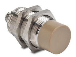
AutomationDirect inductive proximity sensor, tubular, 30mm diameter x 70mm body, 316L stainless steel housing, N.O. output, 22mm sensing distance, non-flush, 25 Hz (AC)/100 Hz (DC) switching frequency, IP68 IP69K, 1/2in - 20UNF thread.
