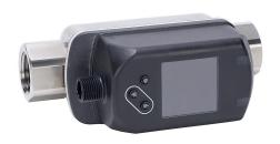
ProSense liquid flow sensor, vortex, 1/2in female NPT process connection, 0.26 to 5.28 GPM, 16 to 317 GPH, 14 to 194 deg F, Output: analog, Output 2: analog, 18-30 VDC operating voltage.
