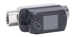
ProSense liquid flow sensor, vortex, 1/2in female NPT process connection, 0.55 to 10.55 GPM, 32 to 634 GPH, 14 to 194 deg F, Output: analog, Output 2: analog, 18 to 30 VDC operating voltage.
