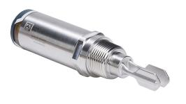
ProSense vibration fork liquid level switch, any orientation mount, 1.89in insertion length, 316L stainless steel wetted parts, -40 to 302 deg F, 3/4in male NPT process connection, switch PNP, 3-wire, N.O./N.C. complementary, 4-pin M12 quick-disconnect.
