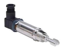
ProSense vibration fork liquid level switch, any orientation mount, 1.89in insertion length, 316L stainless steel wetted parts, -40 to 302 deg F, 3/4in male NPT process connection, switch PNP, 3-wire, N.O. or N.C., EN 175301-803-A connector.
