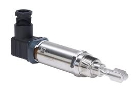
ProSense vibration fork liquid level switch, any orientation mount, 1.89in insertion length, 316L stainless steel wetted parts, -40 to 302 deg F, 3/4in male NPT process connection, AC/DC, 2-wire, N.O. or N.C., EN 175301-803-A connector.
