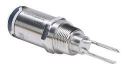
ProSense vibration fork liquid level switch, any orientation mount, 1.89in insertion length, 316L stainless steel wetted parts, -40 to 212 deg F, 3/4in male NPT process connection, switch PNP, 3-wire, N.O./N.C. complementary, 4-pin M12 quick-disconnect.
