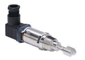
ProSense vibration fork liquid level switch, any orientation mount, 1.89in insertion length, 316L stainless steel wetted parts, -40 to 212 deg F, 3/4in male NPT process connection, switch PNP, 3-wire, N.O. or N.C., EN 175301-803-A connector.
