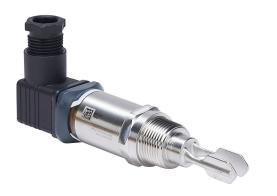
ProSense vibration fork liquid level switch, any orientation mount, 1.89in insertion length, 316L stainless steel wetted parts, -40 to 212 deg F, 3/4in male NPT process connection, AC/DC, 2-wire, N.O. or N.C., EN 175301-803-A connector.
