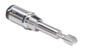
ProSense vibration fork liquid level switch, any orientation mount, 3.44in insertion length, 316L stainless steel wetted parts, -40 to 212 deg F, 3/4in male NPT process connection, switch PNP, 3-wire, N.O./N.C. complementary, 4-pin M12 quick-disconnect.
