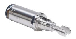
ProSense vibration fork liquid level switch, any orientation mount, 1.89in insertion length, 316L stainless steel wetted parts, -40 to 302 deg F, 1/2in male NPT process connection, switch PNP, 3-wire, N.O./N.C. complementary, 4-pin M12 quick-disconnect.
