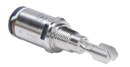
ProSense vibration fork liquid level switch, any orientation mount, 1.89in insertion length, 316L stainless steel wetted parts, -40 to 212 deg F, 1/2in male NPT process connection, switch PNP, 3-wire, N.O./N.C. complementary, 4-pin M12 quick-disconnect.
