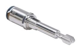
ProSense vibration fork liquid level switch, any orientation mount, 3.44in insertion length, 316L stainless steel wetted parts, -40 to 212 deg F, 1/2in male NPT process connection, switch PNP, 3-wire, N.O./N.C. complementary, 4-pin M12 quick-disconnect.
