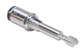
ProSense vibration fork liquid level switch, any orientation mount, 3.44in insertion length, 316L stainless steel wetted parts, -40 to 212 deg F, 1/2in male NPT process connection, switch PNP, 3-wire, N.O./N.C. complementary, 4-pin M12 quick-disconnect.
