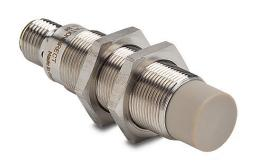
AutomationDirect inductive proximity sensor, tubular, 18mm diameter x 70mm body, 316L stainless steel housing, N.O. output, 12mm sensing distance, non-flush, 25 Hz (AC)/300 Hz (DC) switching frequency, IP68 IP69K, 1/2in - 20UNF thread.
