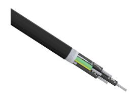
Southwire flexible VFD/Servo cable, shielded, 4 conductors (includes ground), 16 AWG, 26-stranded, tinned copper, (1) shielded 16 AWG twisted pair, XLPE conductor insulation material, TPE jacket, black, cut to length.
