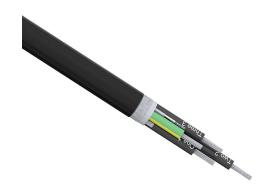
Southwire flexible VFD/Servo cable, shielded, 4 conductors (includes ground), 14 AWG, 41-stranded, tinned copper, (1) shielded 16 AWG twisted pair, XLPE conductor insulation material, TPE jacket, black, cut to length.
