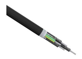
Southwire flexible VFD/Servo cable, shielded, 4 conductors (includes ground), 12 AWG, 65-stranded, tinned copper, (1) shielded 16 AWG twisted pair, XLPE conductor insulation material, TPE jacket, black, cut to length.
