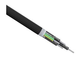
Southwire flexible VFD/Servo cable, shielded, 4 conductors (includes ground), 10 AWG, 105-stranded, tinned copper, (1) shielded 16 AWG twisted pair, XLPE conductor insulation material, TPE jacket, black, cut to length.
