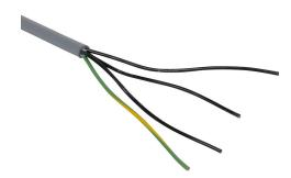
Southwire flexible control cable, unshielded, 4 conductors (includes ground), 10 AWG, bare copper, PVC/Nylon conductor insulation material, black with white numbers and green/yellow ground, TPE jacket, gray, cut to length.
