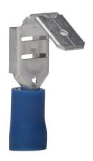
Z+F piggy back disconnect, 16-14 AWG, blue, 6.3 x 0.8mm tab size, partially PVC insulated. Package of 100.
