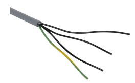
Southwire flexible control cable, unshielded, 4 conductors (includes ground), 12 AWG, bare copper, PVC/Nylon conductor insulation material, black with white numbers and green/yellow ground, TPE jacket, gray, cut to length.
