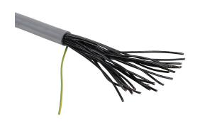
Southwire flexible control cable, unshielded, 25 conductors (includes ground), 14 AWG, bare copper, PVC/Nylon conductor insulation material, black with white numbers and green/yellow ground, TPE jacket, gray, cut to length.
