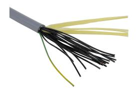
Southwire flexible control cable, unshielded, 18 conductors (includes ground), 14 AWG, bare copper, PVC/Nylon conductor insulation material, black with white numbers and green/yellow ground, TPE jacket, gray, cut to length.
