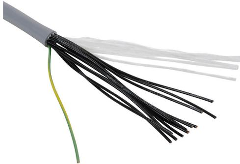
Southwire flexible control cable, unshielded, 12 conductors (includes ground), 14 AWG, bare copper, PVC/Nylon conductor insulation material, black with white numbers and green/yellow ground, TPE jacket, gray, cut to length.
