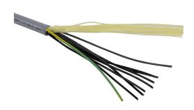
Southwire flexible control cable, unshielded, 9 conductors (includes ground), 14 AWG, bare copper, PVC/Nylon conductor insulation material, black with white numbers and green/yellow ground, TPE jacket, gray, cut to length.
