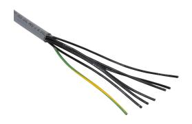
Southwire flexible control cable, unshielded, 7 conductors (includes ground), 14 AWG, bare copper, PVC/Nylon conductor insulation material, black with white numbers and green/yellow ground, TPE jacket, gray, cut to length.
