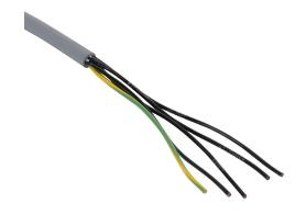
Southwire flexible control cable, unshielded, 5 conductors (includes ground), 14 AWG, bare copper, PVC/Nylon conductor insulation material, black with white numbers and green/yellow ground, TPE jacket, gray, cut to length.
