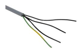
Southwire flexible control cable, unshielded, 4 conductors (includes ground), 14 AWG, bare copper, PVC/Nylon conductor insulation material, black with white numbers and green/yellow ground, TPE jacket, gray, cut to length.
