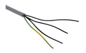
Southwire flexible control cable, unshielded, 4 conductors (includes ground), 14 AWG, bare copper, PVC/Nylon conductor insulation material, black with white numbers and green/yellow ground, TPE jacket, gray, cut to length.
