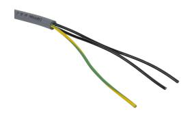
Southwire flexible control cable, unshielded, 3 conductors (includes ground), 14 AWG, bare copper, PVC/Nylon conductor insulation material, black with white numbers and green/yellow ground, TPE jacket, gray, cut to length.
